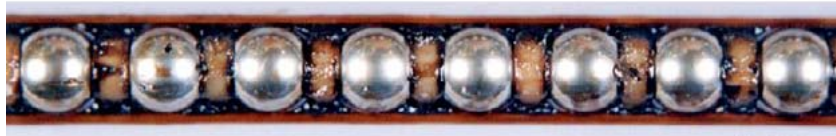
Ball cage after running 8,000 km Nominal life: L_{10} = 400 km Remaining grease is observed in the ball cage. 5 mm
