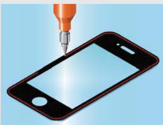
Sealant dispensing of PUR for smartphone's cover
