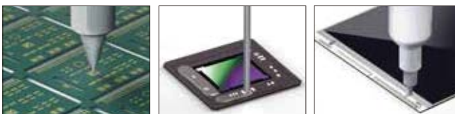
Ag paste dispensing for die bonding
