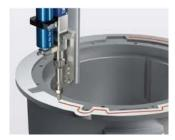
High speed positive displacement dispenser ideal for use with liquid gasket materials
