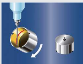
Dispensing of 2-part epoxy adhesive to motors
