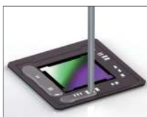
Dust trapping agent dispensing on camera modules
